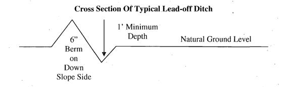
All lead-off ditches shall be graded to drain water with a 1 percent minimum to 3 percent maximum ditch slope. The spacing interval are variable for lead-off ditches and shall be determined according to the formula for spacing intervals of lead-off ditches, but may be amended depending upon existing soil types and centerline road slope (in %);
