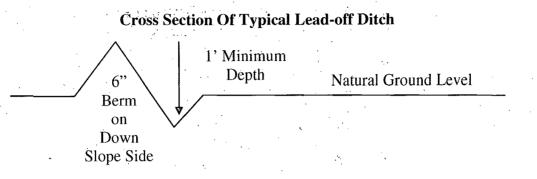
All lead-off ditches shall be graded to drain water with a 1 percent minimum to 3 percent maximum ditch slope. The spacing interval are variable for lead-off ditches and shall be determined according to the formula for spacing intervals of lead-off ditches, but may be amended depending upon existing soil types and centerline road slope (in %);
