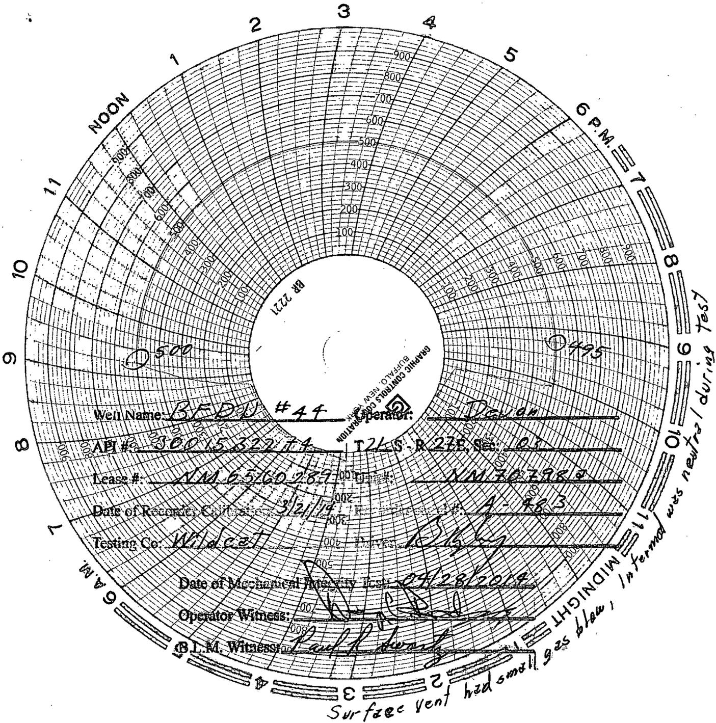
Surface vent had small gas blow, internal was neutral during test
