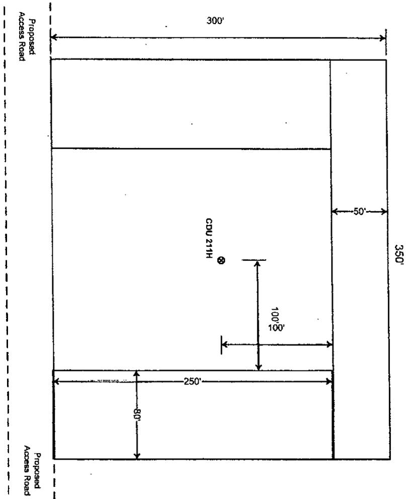
Note: A distance of 100' is required between fired vessels and any combustibles for safety purposes.
