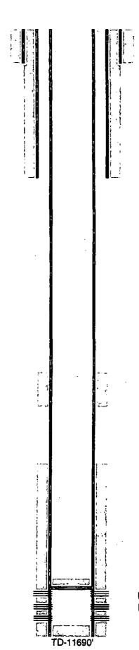
17-1/2" hole @ 600' 13-3/8" csg @ 600' w/ 1075sx-TOC-Surf-Circ
