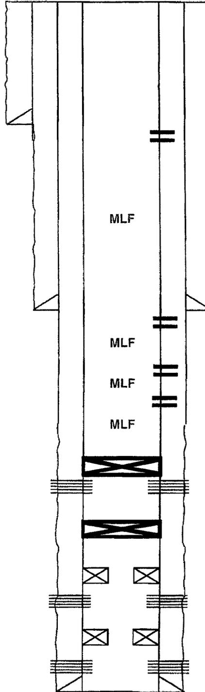
**PERF@650' AND SQUEEZE 200SX OF CLASS "C" CEMENT FROM FROM 650'-SURFACE. WOC & TAG.**
