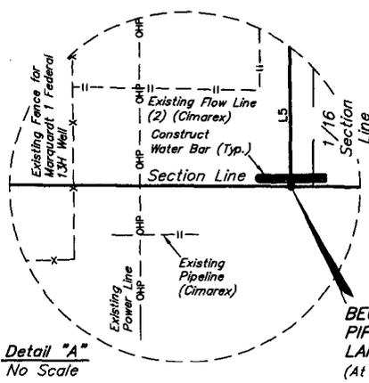
BEGINNING OF PROPOSED GAS SALES PIPELINE RIGHT-OF-WAY ON BLM LANDS IN SEC. 1 STA. 25+97.89 (At Section Line)
