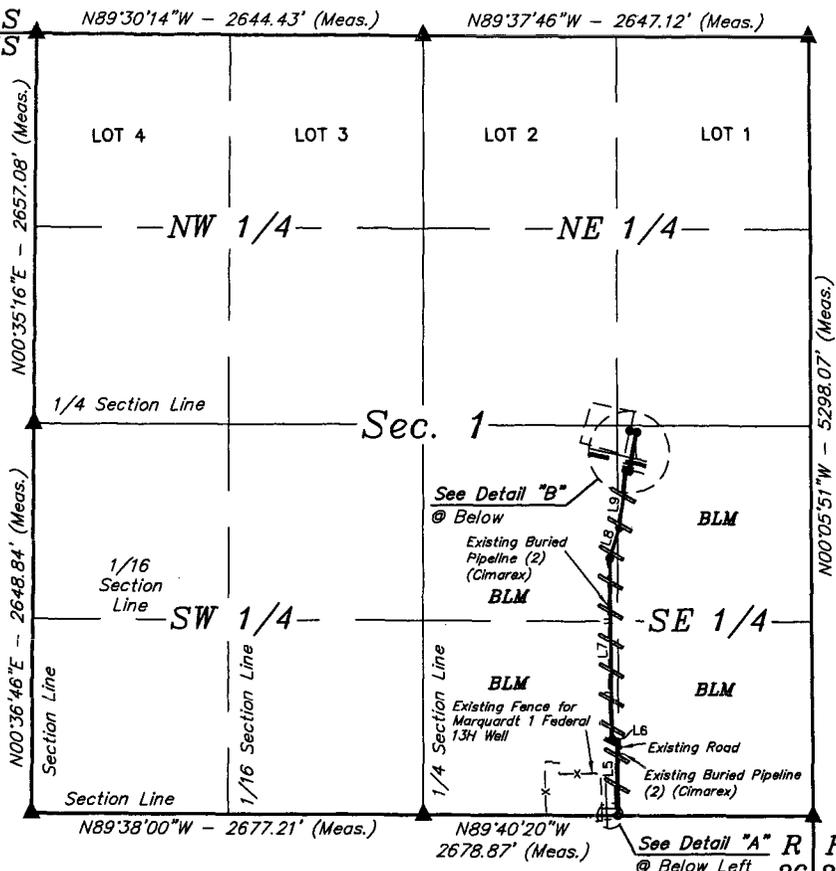
END OF PROPOSED GAS SALES PIPELINE RIGHT-OF-WAY STA. 53+17.67 (At Edge of Existing Aqueduct Compressor Station)
