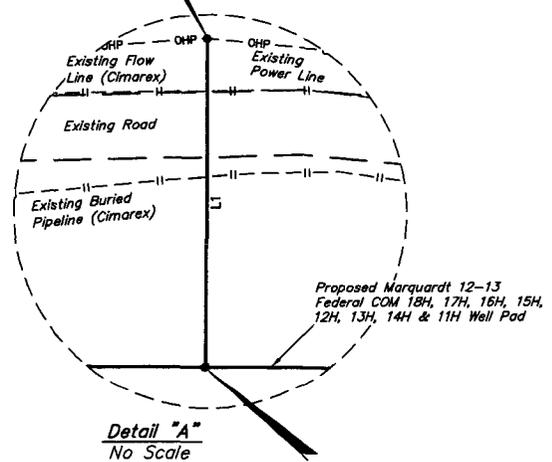
END OF PROPOSED POWER LINE RIGHT-OF-WAY STA. 1+51.52 (At Edge of Proposed Marquardt 12-13 Federal COM 18H, 17H, 16H, 15H, 12H, 13H, 14H & 11H Well Pad)
