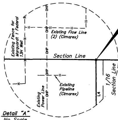
**END OF PROPOSED GAS SALES PIPELINE RIGHT-OF-WAY ON BLM LANDS IN SEC. 12 STA. 25+97.89 (At Section Line)**
