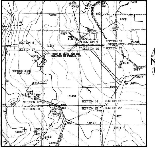
SEC. 17 TWP. 23-S RGE. 27-E SURVEY: N.M.P.M. COUNTY: EDDY DESCRIPTION: 1649' FNL & 315' FEL ELEVATION: 3164' OPERATOR: MARATHON OIL PERMIAN, LLC LEASE: CASS 16 STATE U.S.G.S. TOPOGRAPHIC MAP: OTIS, N.M.
