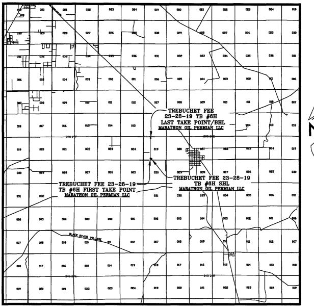
SEC. 19 TWP. 23-S RGE. 28-E SURVEY: N.M.P.M. COUNTY: EDDY DESCRIPTION: 270' FSL & 1878' FWL ELEVATION: 3084' OPERATOR: MARATHON OIL PERMIAN LLC LEASE: TREBUCHET FEE 23-28-19 U.S.G.S. TOPOGRAPHIC MAP: OTIS, N.M. SCALE: 1" = 2 MILES
