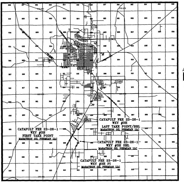
SEC. 1 TWP. 23-S RGE. 26-E SURVEY: N.M.P.M. COUNTY: EDDY DESCRIPTION: 463' FSL & 1527' FEL ELEVATION: 3219' OPERATOR: MARATHON OIL PERMIAN LLC LEASE: CATAPULT FEE 23-26-1 U.S.G.S. TOPOGRAPHIC MAP: OTIS, N.M. SCALE: 1" = 2 MILE
