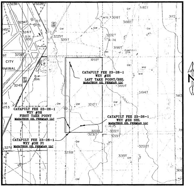
SEC. 1 TWP. 23-S RGE. 26-E SURVEY: N.M.P.M. COUNTY: EDDY DESCRIPTION: 463' FSL & 1527' FEL ELEVATION: 3219' OPERATOR: MARATHON OIL PERMIAN LLC LEASE: CATAPULT FEE 23-26-1 U.S.G.S. TOPOGRAPHIC MAP: OTIS, N.M.
