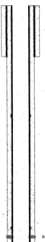
12-1/4" hole @ 1797' 9-5/8" csg @ 1785' w/ 1225sx-TOC-Surf-Circ
