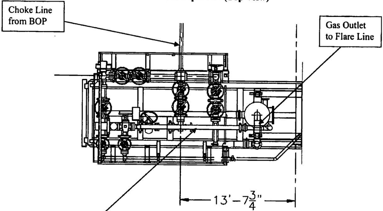
**Choke Manifold – Gas Separator (Side View)**
