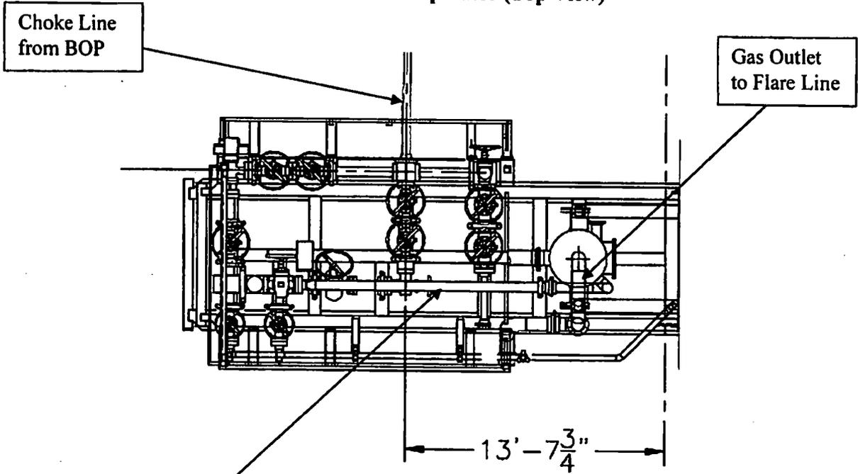
**Choke Manifold – Gas Separator (Side View)**
