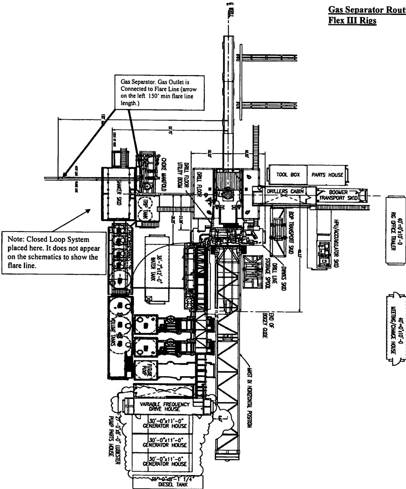
**Choke Manifold – Gas Separator (Top View)**
