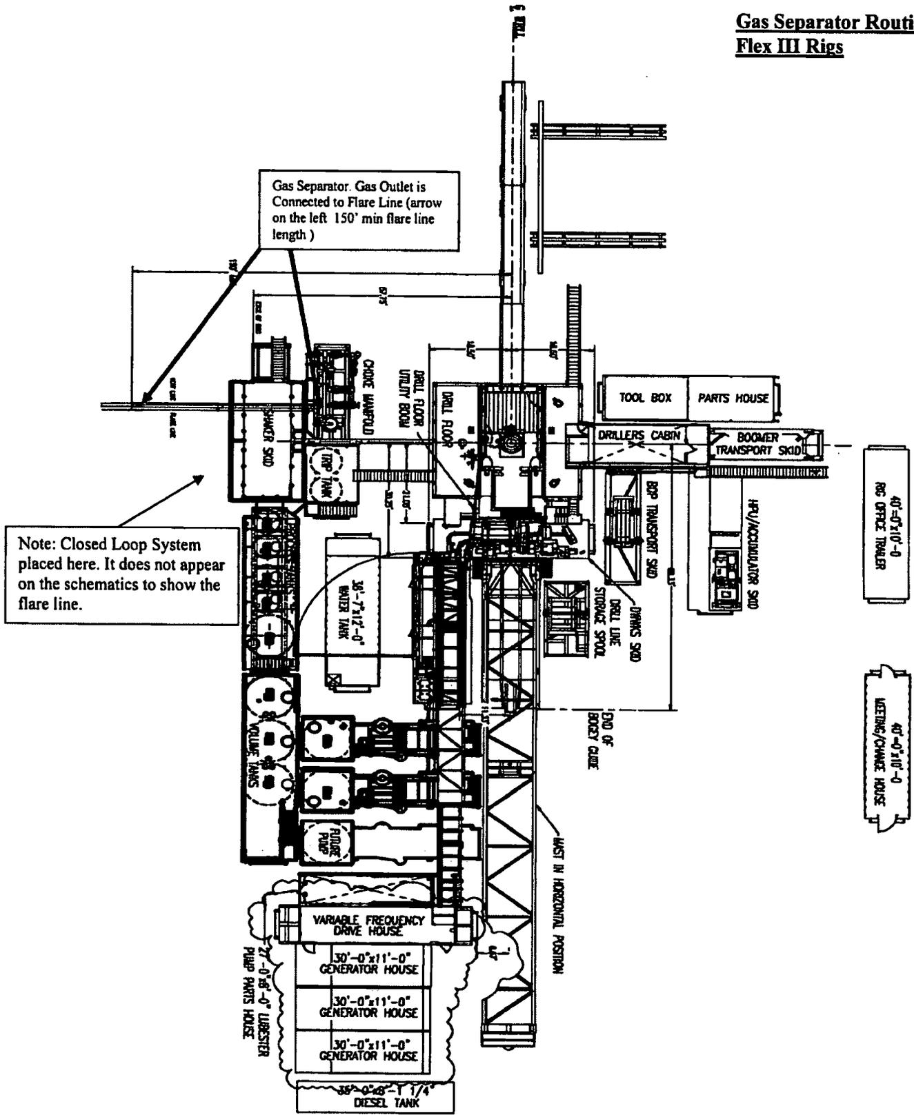
**Choke Manifold – Gas Separator (Top View)**
