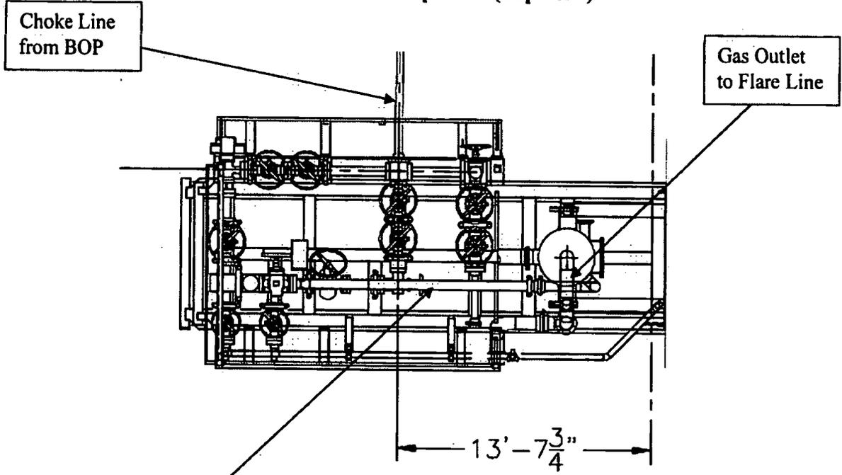
**Choke Manifold – Gas Separator (Side View)**
