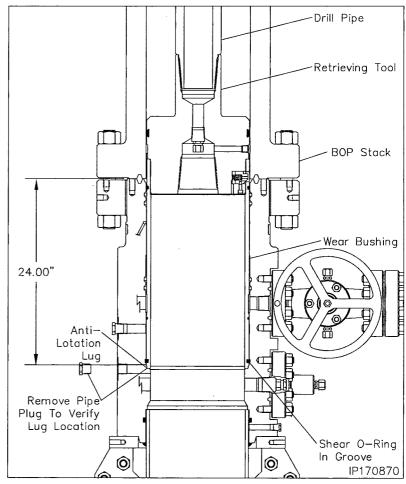
**Note:** The Shear O-Ring on bottom of the bushing will locate in a groove above the load shoulder in the head to act as a retaining device for the bushing.
