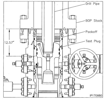
Remove as much fluid as possible from the BOP stack and the retrieve the test plug with a straight vertical
