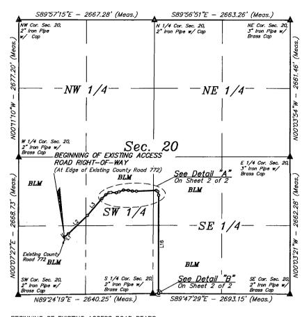
LINE TABLE LINE DIRECTION LENGTH L1 N50'40'57"E 96.65 12 N46'35'31"E 517.21 L3 N40'47'31"E 427.52 N45°21'07"E 14 111.07 15 N57°57'47"E 73.15 16 N83'07'18"E 41.28 17 S86'28'22"E 103.30 N70°53'43"E 55.57 18 L9 N6817'28"E 93.53 L10 S86\*56'51"E 94.80 L11 S80"01'31"E 82.01 L12 S87'34'28"E 78.98 L13 N87'32'13"E 388.41 L14 S53"20"02"E 39.17 L15 S14'43'41"E 71.27 L16 S00'03'00"E 1889.06 L17 S04'01'34"E 18.99'
