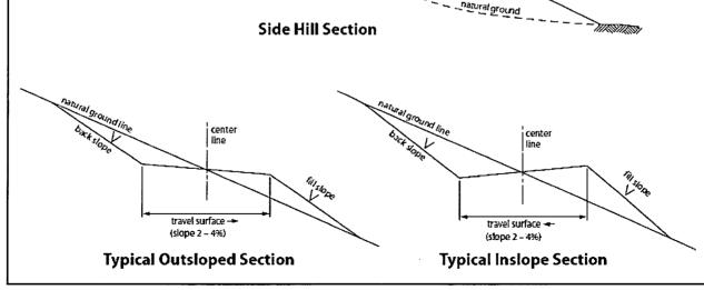
Figure 1. Cross-sections and plans for typical road sections representative of BLM resource or FS local and higher-class roads.
