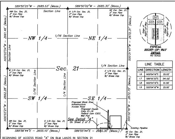
BEGINNING OF ACCESS ROAD "A" ON BLM LANDS IN SECTION 21 BEARS N89'55'44"W 1168.61' FROM THE SOUTHEAST CORNER OF SECTION 21, T24S, R26E, N.M.P.M.
