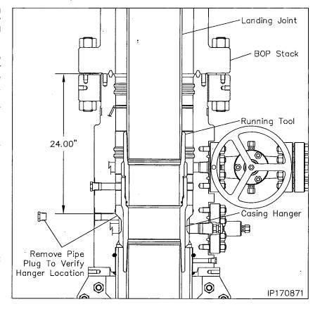
26. <u>Using Chain Tongs Only located</u> 180° apart, retrieve the Running Tool and landing joint by rotating the landing joint clockwise (right) approximately 16 turns.
