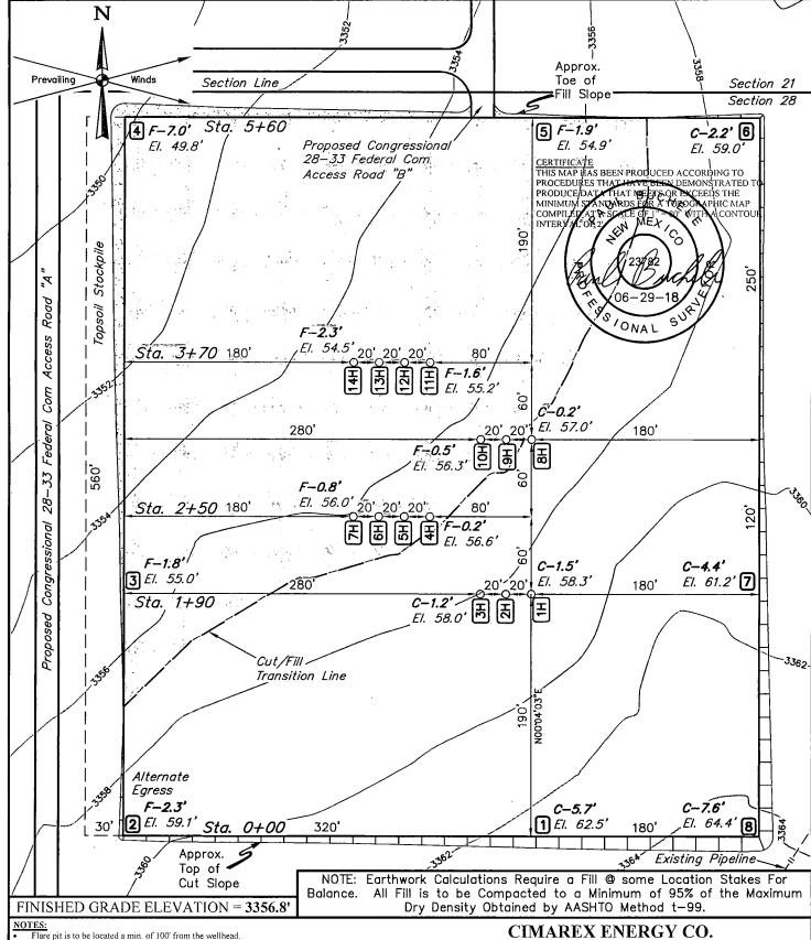
Flare pit is to be located a min. of 100' from the wellhead.
