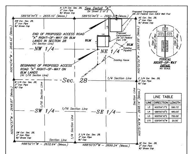
BEGINNING OF ACCESS ROAD "A" ON BLM LANDS BEARS S36'57'59"E 1679.60' FROM THE NORTH 1/4 CORNER OF SECTION 28, T24S, R26E, N.M.P.M.
