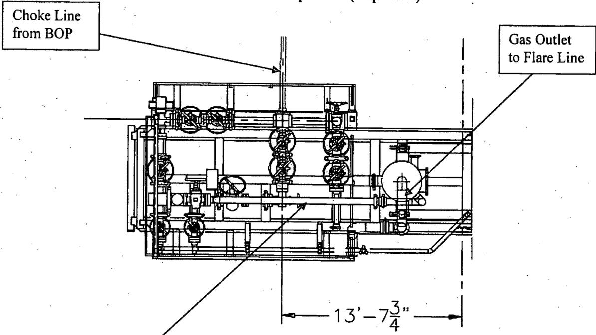
**Choke Manifold – Gas Separator (Side View)**
