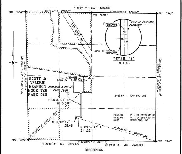
A strip of land 30 feet wide, being 1,265.87 feet or 76.719 rods in length, lying in Section 23, Township 24 South, Range 28 East, N. M. P. M., Eddy County, New Mexico, being 15 feet left and 15 feet right of the following described survey of a centerline across the lands of Scott and Valerie Branson, according to a deed filed for record in Book 728, Page 526, of the deed records of Eddy County, New Mexico:
