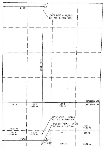
NAD 83 NME <u>SURFACE LOCATION</u> Y=364249.5 N X=647661.3 E LAT.=32.000938 N LONG.=103.990338 W BOREPATH SHOWN HEREON IS BASED ON DIRECTIONAL SURVEY REPORT PROVIDED BY COG OPERATING, LLC FOR THE LITTLEFIELD 33 FEDERAL COM #705H SUPPLIED TO HARCROW SURVEYING, LLC ON JUNE 5, 2019
