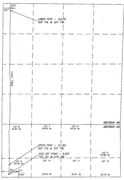
NAD 83 NME SURFACE LOCATION Y=364195.1 N X=645976.3 E LAT.=32.000803' N LONG.=103.995774° W BOREPATH SHOWN HEREON IS BASED ON DIRECTIONAL SURVEY REPORT PROVIDED BY COG OPERATING, LLC FOR THE LITTLEFIELD 33 FEDERAL COM #708H SUPPLIED TO HARCROW SURVEYING, LLC ON JUNE 5, 2019
