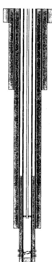
17-1/2" hole @ 715' 13-3/8" csg @ 715' w/ 830sx-TOC-Surf-Circ.
