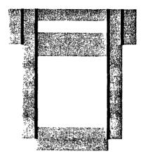
17-1/2" hole @ 407' 13-3/8" csg @ 407' w/363sx-TOC-Surf-Circ
