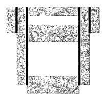
17-1/2" hole @ 436' 13-3/8" csg @ 436' w/400sx-TOC-Surf-Circ
