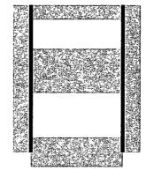
12-1/4" hole @ 1530' 9-5/8" csg @ 1530' w/ 1955sx-TOC-Surf-Circ
