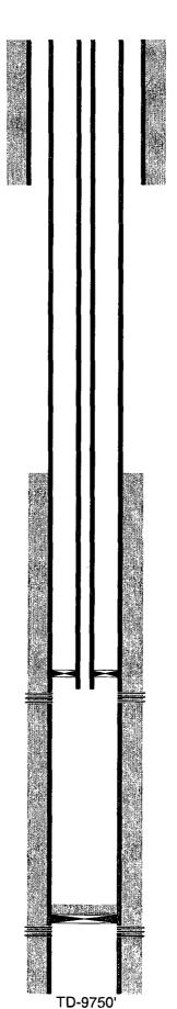
12-1/4" hole @ 1500' 8-5/8" csg @ 1500' w/1030sx-TOC-Surf-Circ
