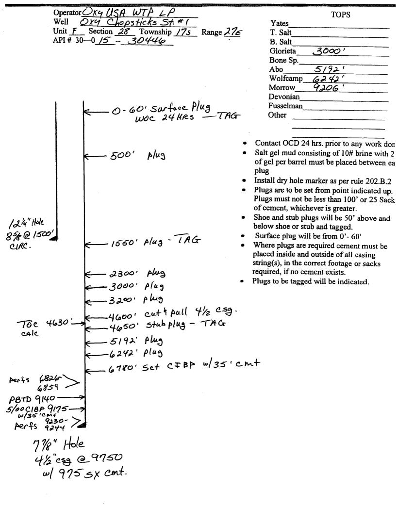
**OXY USA WTP LP - Proposed** 20sx Surface 0-60' Surface Plug-WOC24HRS-TAG/TOPOFF CM+
