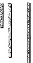
16" Conductor Casing Set @ 40'. Cemented to Surface w/ Redi-Mix
