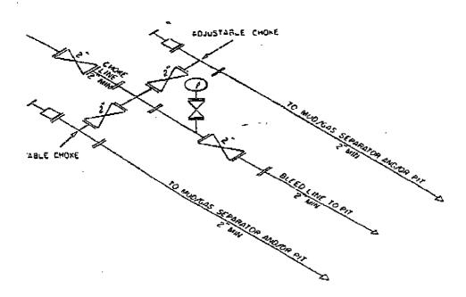
2M CHOKE MANIFOLD EQUIPMENT — CONFIGURATION OF CHOKES STAY VARY
