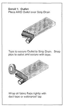
Detail 1: Use outlet (product FO.06) as shown to connect strip drain to Perforated FlexDrain with Sock. Use FlexDrain to connect drainage mats together or to connect to riser pipes.
