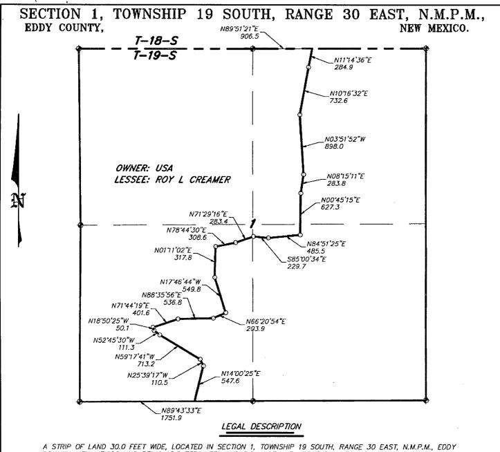
A STRIP OF LAND 30.0 FEET WIDE, LOCATED IN SECTION 1, TOWNSHIP 19 SOUTH, RANGE 30 EAST, N.M.P.M., EDDY COUNTY, NEW MEXICO AND BEING 15.0 FEET LEFT AND RIGHT OF THE ABOVE PLATTED CENTERLINE SURVEY.
