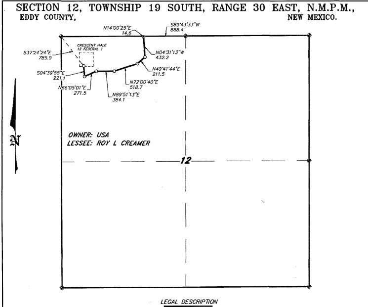
A STRIP OF LAND 30.0 FEET WIDE, LOCATED IN SECTION 12, TOWNSHIP 19 SOUTH, RANGE 30 EAST, N.M.P.M., EDDY COUNTY, NEW MEXICO AND BEING 15.0 FEET LEFT AND RIGHT OF THE ABOVE PLATTED CENTERLINE SURVEY.
