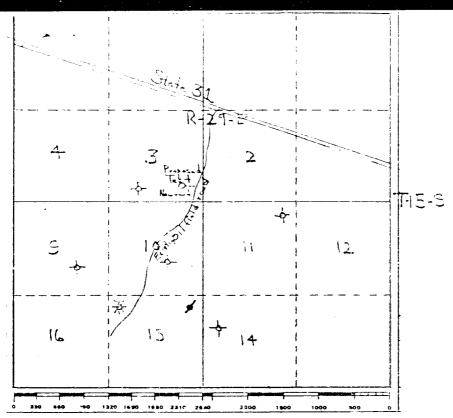
PROPOSE TO USE EXISTING ROADS, OIL FIF'D AND RANCH, AND TO CONSTRUCT APPROXIMATELY 300" OF NEW ROAD TO LOCATION. NO WATER IN SUFFICIENT QUANTITIES EXISTS IN THIS AREA AND WILL HAVE TO BE TRUCKED TO LOCATION. COMBUSTIBLE MATERIAL WILL BE BURNED. NONCOMBUSTIBLE MATERIAL WILL BE BURNED WITH PIT FILLING.
