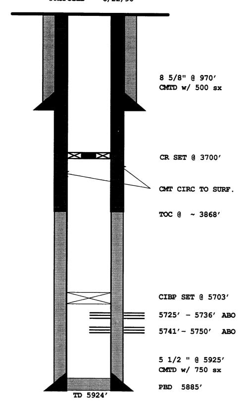
NOTE: There is no record of the cement top on the production casing. Calculated values are as follows:
