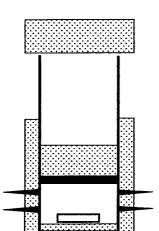
CEMENT PLUG: 5276'- 5408' WITH 35 SXS CUT-OFF 4 1/2" CASING @ 5428'
