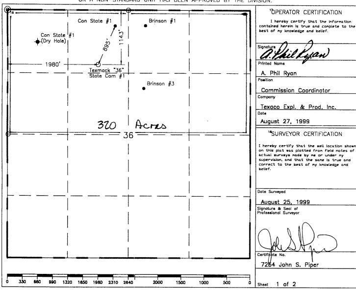
O = Staked Location • = Producing Well 🔎 = Injection Well 💀 = Water Supply Well 🔶 = Plugged & Abandon Well ○ = Found Section Corner, 2 or 3" Iron Pipe & GLO B.C.
