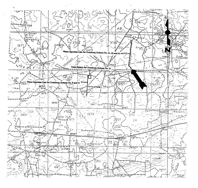
Figure 1. Showing BURNETT OIL COMPANY, INC.'S proposed Grayburg Jackson Well No. 21 Tank Battery Pad; (approx. 250' X 200'); Water Injection Line serving the Grayburg Jackson Well No. 8 and 21, (150' X approx. 1800'); and Water Injection Line serving the Grayburg Jackson Well No. 41, 26, and 31; (150' X approx. 2700'); in Sections 23, 14, and 13, T17S, R30E, NMPM, Eddy County, NM Map Reference: USGS 7.5' Series, Loco Hills, NM (1985 Prov. Ed.)
