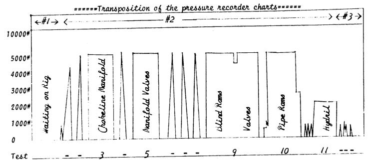
The above is a transposition of the pressure recorder charts covering test to the blowout control equipment in service on your well drilling in the Loco Hills, New Mexico Area, Midland District, Texas. Test was made with test plug landed in casing head with the following test results:
