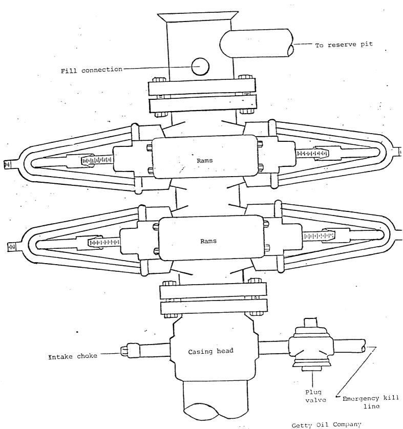
5000 psi working pressure Drilling control hookup
