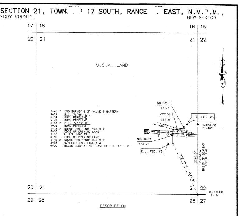
A STRIP OF LAND 50.0 FEET WIDE, 848.7 FEET OR 0.161 MILES IN LENGTH AND BEING 25.0 FEET LEFT AND 25.0 FEET RIGHT OF THE ABOVE CENTERLINE SURVEY.
