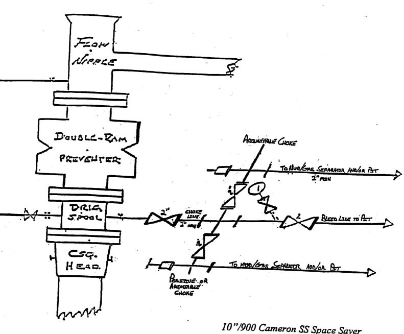
Marbob Energy Corporation Foran State No. 2 1650' FNL & 330' FEL Section 16; T17s – R31e Eddy County, New Mexico 10"/900 Cameron SS Space Saver 3000# Working Pressure 3000# Working Pressure Choke Manifold DISTRICT I P.O. Box 1980, Hobbs, NM 88241-1980 State of New Mexico
