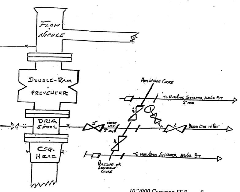
10"/900 Cameron SS Space Saver 3000# Working Pressure 3000# Working Pressure Choke Manifold
