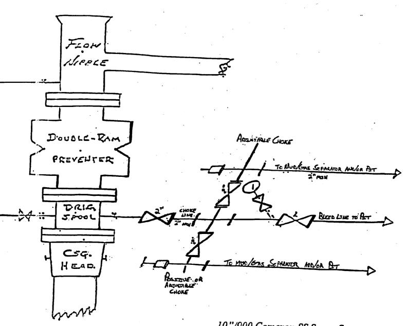
10"/900 Cameron SS Space Saver 3000# Working Pressure 3000# Working Pressure Choke Manifold
