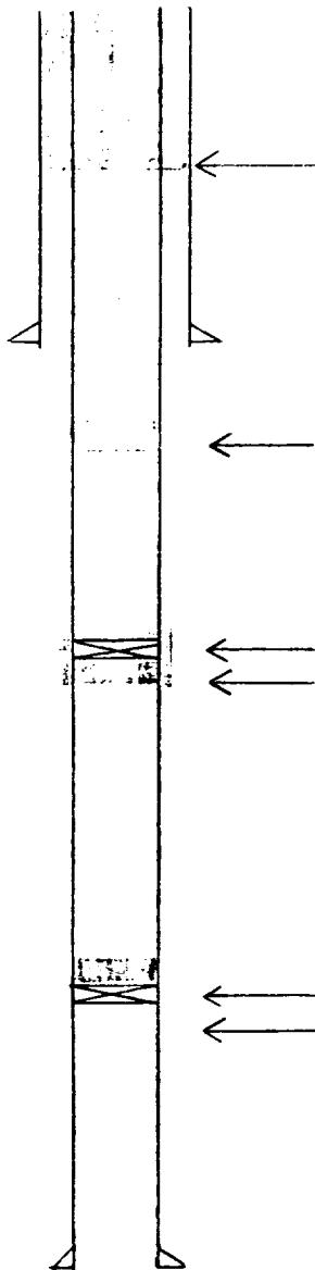
Perforations @ 400' w/4 holes per foot in 7" casing
