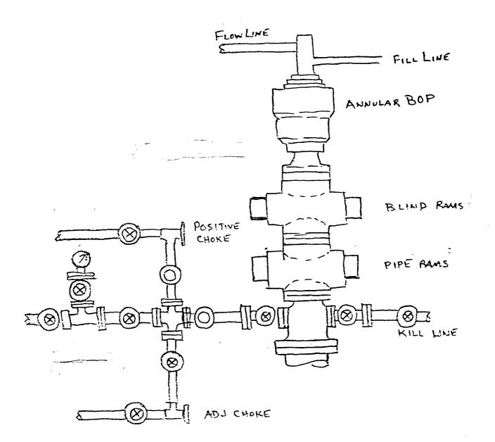
This 10" - 3000 W.P. stack is to be nippled up on the 13 3/8 csg and used while drilling 300'- 2800'.
