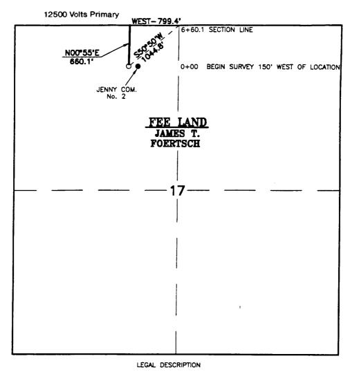
A STRIP OF LAND 30.0 FEET WIDE, LOCATED IN SECTION 17, TOWNSHIP 19 SOUTH, RANGE 25 EAST, N.M.P.M., EDDY COUNTY, NEW MEXICO AND BEING 15.0 FEET LEFT AND RIGHT OF THE FOLLOWING DESCRIBED CENTERLINE SURVEY.
