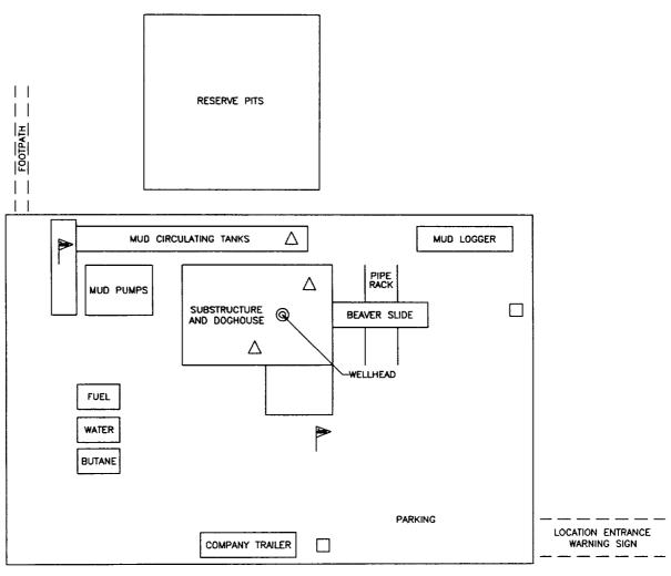
H2S MONITORS WITH ALARMS AT THE BELL NIPPLE, SUBSTRUCTURE, AND SHALE SHAKER
