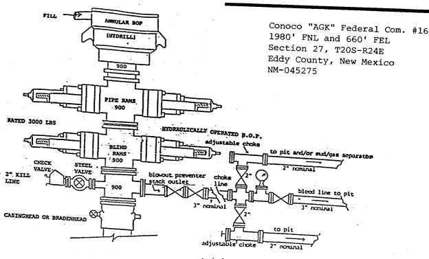
typical choke manifold assemby for 14 rated working pressure service-surface installation
