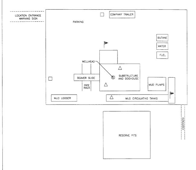
$\triangle$  H2S MONITORS WITH ALARMS AT THE BELL NIPPLE, SUBSTRUCTURE, AND SHALE SHAKER WIND DIRECTION INDICATORS
