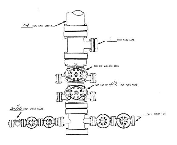
\*\*OTE: ALL VALVES ARE METAL-TO-METAL SEAL AND FLANGED. ALL COMPONENTS MUST MEET ABOVE MINIMAM PRESSURE RATIMSS. ALL COMPONENTS TO BE TESTED TO RATED PRESSURE AFTER ASSEMBLY AND BEFORE FURTHER DOWN-DUE OPERATIONS MAY BE CONDUCTED.
