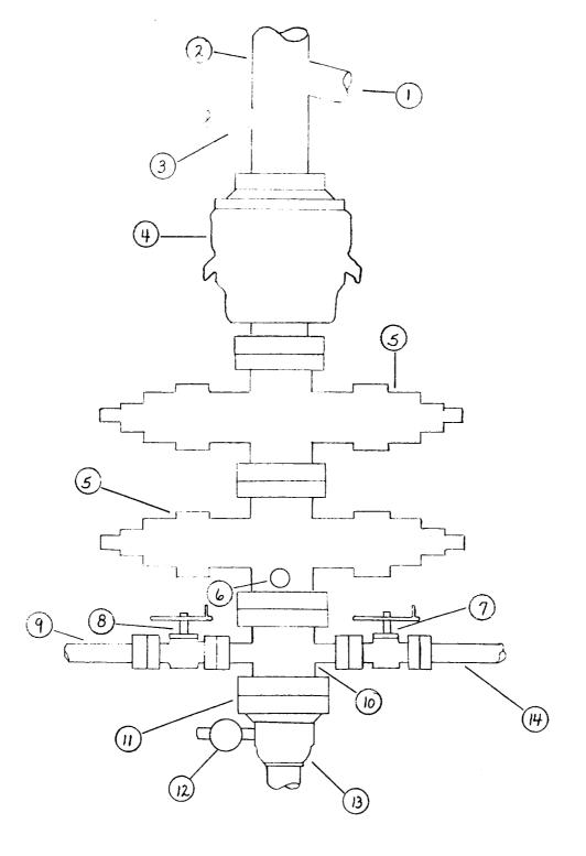
BOP will be installed after 9 5/8" casing is set.
