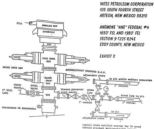
working pressure service-surface installation
