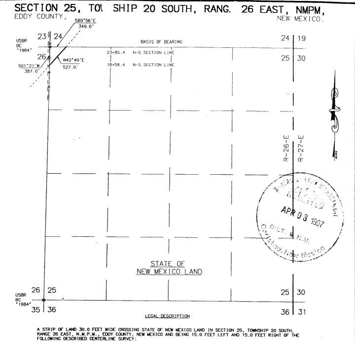
BEGINNING AT A POINT ON THE WEST LINE OF SAID SECTION 25 WHICH LIES SO1°21'W, 387.0 FEET FROM A USBR BRASS CAP FOUND FOR THE THE NORTHMEST CORNER OF SAID SECTION 25; THENCE N42°49'E, 527.0 FEET TO A POINT ON THE NORTHLINE OF SAID SECTION 25 WHICH LIES S89°56'E, 349.0 FEET FROM SAID NORTHWEST CORNER OF SAID SECTION 25. SAID STRIP OF LAND BEING 527.0 FEET OR 31.94 RODS IN LENGTH AND CONTAINS 0.363 ACRES MORE OR LESS AND BEING ALLOCATED BY FORTIES AS FOLLOWS:
