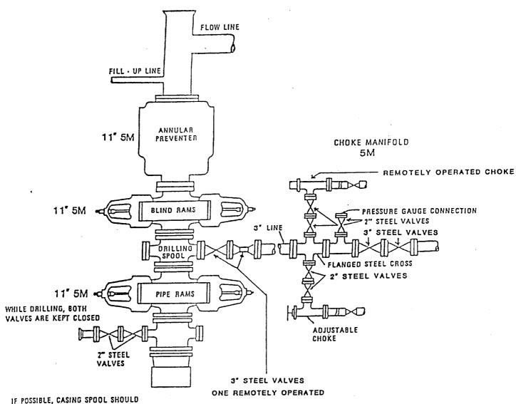
IF POSSIBLE, CASING SPOOL SHOULD BE POSITIONED SO THAT THESE VALVES ARE DIRECTLY UNDER THE BARREL OF THE RAM PREVENTER.
